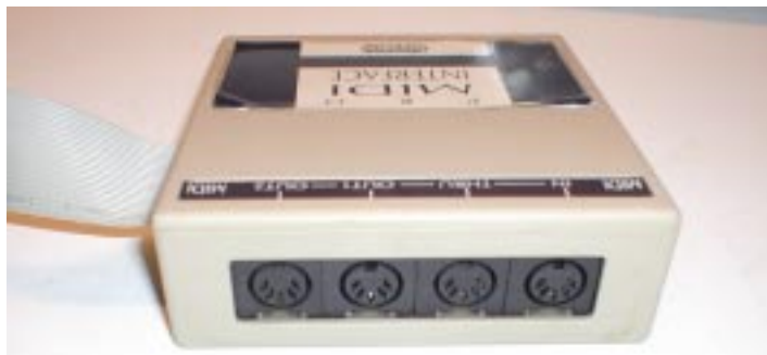
A MIDI interface like this one connects to the Amiga's serial port. MIDI instruments connect to the 5 pin DIN ports.
