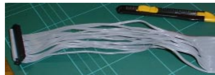
Splitting the cable is easy as long as you take care.
