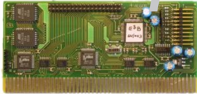
An updated Kickstart for OS 4 can be stored in the flash ROM on several new Zorro cards including E3B's ALGOR USB.
