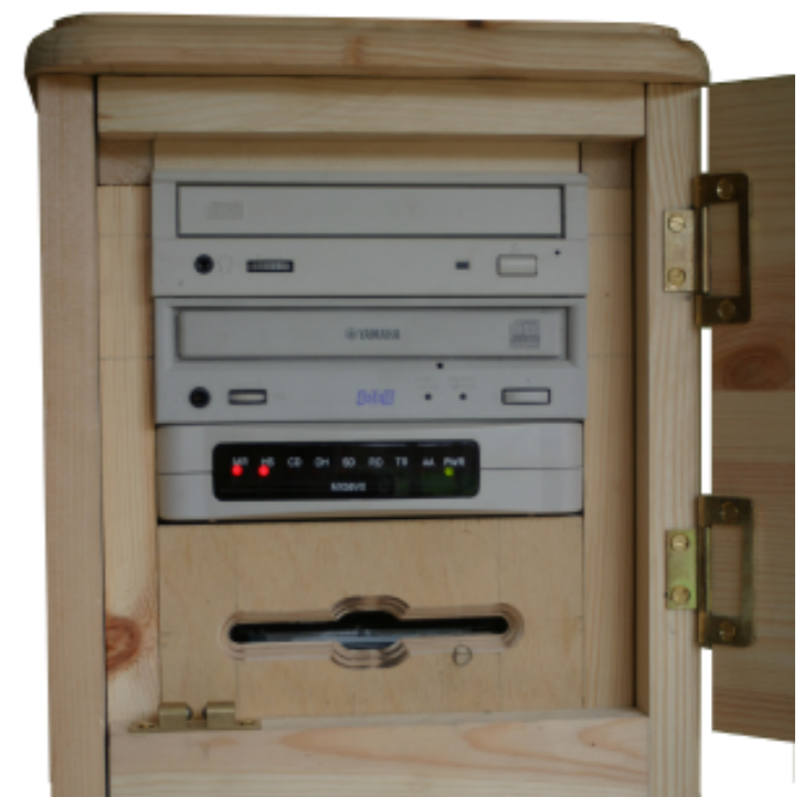
Behind the door, a CD-ROM, CD writer and modem are installed. The floppy drive is behind the neatly routed slot.
